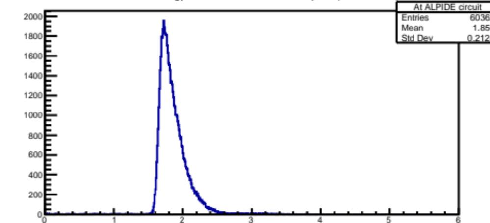
Lossed Energy in ALPIDE epitaxial + substruct at Alpha (d = 14mm)
